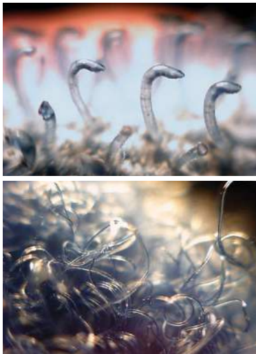
Figure D2: Magnified images of VELCRO® showing the tiny hooks and loops
